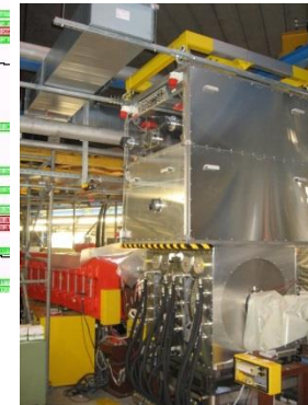
h=2 acceleration cavities for faster ramping
