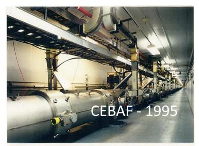
SOUTH LINAC CRYOMODULES
