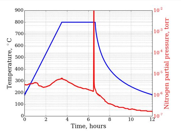
Injection of small nitrogen partial pressure at the end of 800C degassing-> drastic increase in Q
