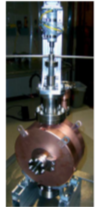
1.3 GHz deflecting cavity @ Cornell
