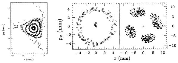
Model-independent analysis of Tevatron turn-by-turn data, including coupling and shifted-BPM constraints [Petrenko et al., PRSTAB **14**, 092801 (2011)]
