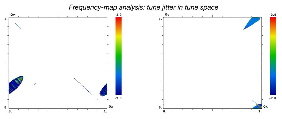
In both cases there are 2 transverse invariants the beam can cross integer resonances without particle loss
