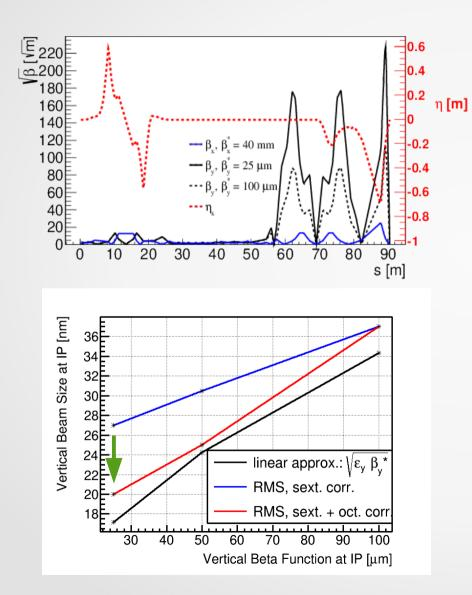
Decreased  $\beta_y^*$  causes the increase of  $\beta_y$  in the Final Focus region. In consequence the beam size is larger in the FF and more sensitive to beam line imperfections. It was checked that:
