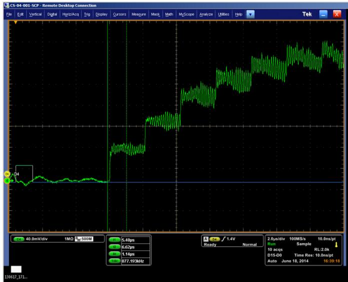
→  $\pi$  orbit bump with linear 80  $\mu$ s fall time, in order to paint the horizontal phase-space
