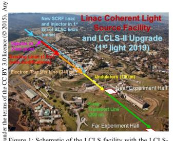
Figure 1: Schematic of the LCLS facility with the LCLSused II SCRF upgrade shown in blue.
