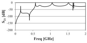
Figure 2:  $S_{21}$  of the HOM filter, with  $TE_{11}$  mode on the hook side and TEM mode on the port side.
