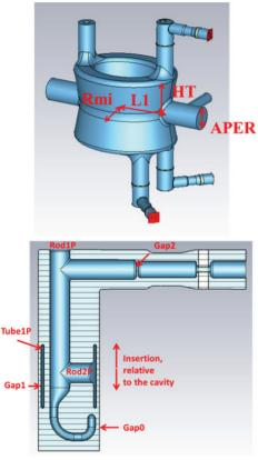
Figure 4: Illustration of the parameters for fabrication error evaluation of the (a) cavity; (b) HOM filter.
