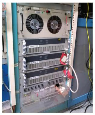
Figure 1: 3 Kepco 10-100GL Units In Parallel.
