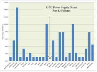
Figure 3: Run 12 Power Supply Failures.
