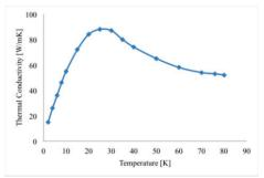
Figure 2: Temperature dependent thermal conductivity of niobium.
