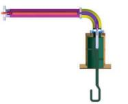
Figure 3: Rigid coaxial line of HOM coupler, showing a section of the connection.
