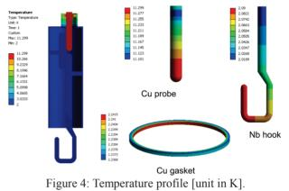
The finite element analysis shows the temperature increase about 0.1 K at the niobium hook extremity, 0.24 K at the copper gasket. The temperature profile was checked against the initial assumption of the temperature dependent surface resistance. The results assure the temperature is converging to a stable point.
