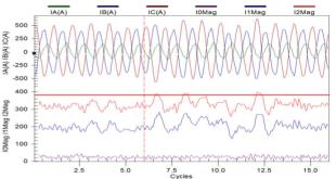
Figure 7: The VVS13 fire phase current and negative sequence current breaker No. 61 sample. The negative sequence current maximum level is market by the red line
