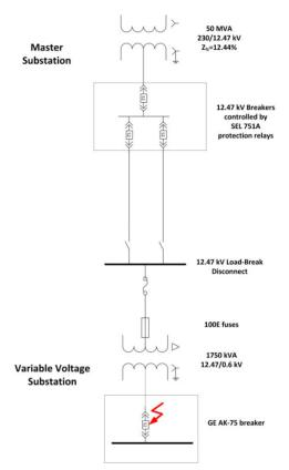
Figure 1: Simplified single line diagram of the VVS substation powering system.
