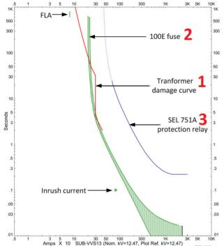
Figure 2: The VVS substation protection coordination graph at the time of the fire. 1 - 12.47 kV transformer damage curve, 2 - 100E fuse, 3 - SEL 751A protection relay overcurrent settings.
