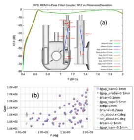
Figure 6. Sensitivity of Q<sub>ext</sub> on coupler dimension errors.
