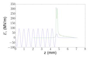
Figure 3: Longitudinal wake generated at the location of the second DLW (blue trace) from corresponding current (green trace). The tail of the bunch corresponds to z < 0.
