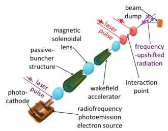
Figure 1: Overview of the compact source scheme: a photoinjected electron bunch passes through a series of DLWs for cascaded acceleration, the resulting high energy electrons are used with a laser to generate inverse Compton scattering.
