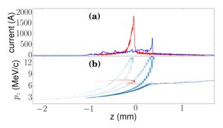
Figure 4: Longitudinal phase space (b) and current projection (a) of before (red) and after (blue) cascaded acceleration. The tail of the bunch corresponds to z < 0.
