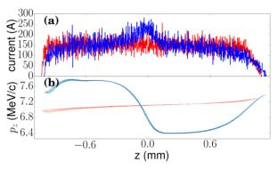
Figure 2: Longitudinal phase spaces (b) and current projection (a) before (red) and after (blue) DLW1 (with parameters listed in Table 1). The tail of the bunch corresponds to z < 0.
