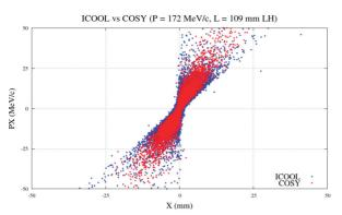
Figure 4: Transverse phase space comparison between COSY (red) and ICOOL (blue).
