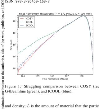
Figure 1: Straggling comparison between COSY (red), G4Beamline (green), and ICOOL (blue).
