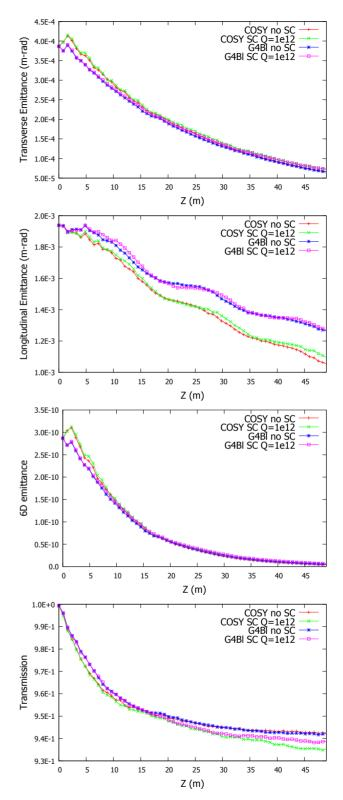
Figure 3: In order from the top, the transverse, longitudinal, 6D emittance, and transmission behavior with and without space charge through 60 cells as simulated in both codes.
