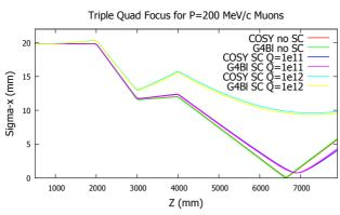
Figure 1: This plot compares the simulated deviation in x of a particle bunch through three quadrupole magnets tuned to focus the muons to a point. For varying amounts of total charge, COSY and G4Beamline are in good agreement.
