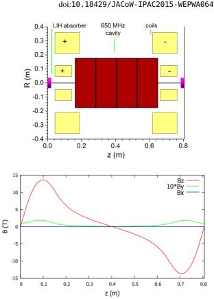
Figure 2: Diagram (top) and magnetic field in the x, y, and z directions (bottom) of a late-stage cooling cell.
