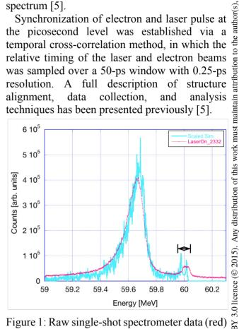
Figure 1: Raw single-shot spectrometer data (red) simulated spectrum (blue), showing evidence of acceleration in the increased width of the smaller peak.
