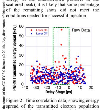
Efigure 2: Time correlation data, showing energy spread of the transmitted electron population versus relative laser-electron timing. Energy modulation is observed near -7 ps for laser-on shots (red) but not laser-off (blue).
