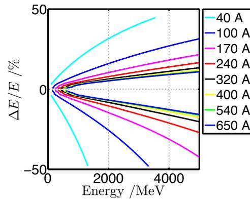
Figure 3:  $\Delta E/E$  vs. energy for dipole HB4 at various magnet current settings.
