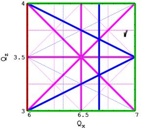
Figure 4: Tune diagram for momenta  $\pm 16\%$  around 3.8 GeV/c. Integer (red), half-integer (green), third integer (blue) and fourth integer (purple) normal resonances are plotted. Structural resonances are in bold.
