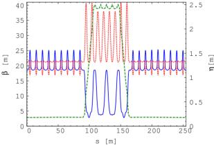
Figure 2: Horizontal (plain blue), vertical (dotted red) periodic betatron functions (left scale) and dispersion (mixed green line, right scale) of half of the ring for matching momentum. The plot is centered on the arc part.
