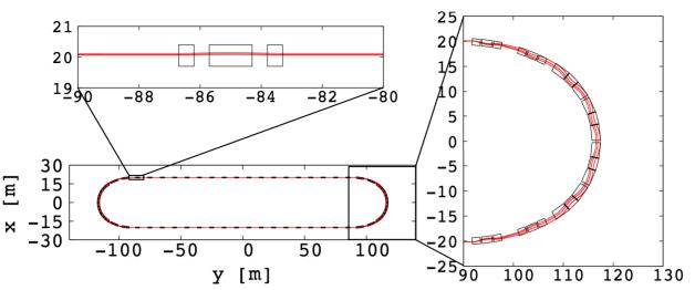
Figure 1: Top view of the racetrack FFAG lattice (bottom left scheme). The top left scheme shows a zoom on the straight section and the right scheme a zoom on the arc section. Matched, minimum and maximum momenta muon closed orbits are shown in red. Effective field boundaries with collimators are shown in black.
