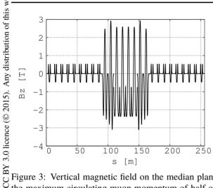
Figure 3: Vertical magnetic field on the median plane for the maximum circulating muon momentum of half of the ring. The plot is centered on the arc part.
