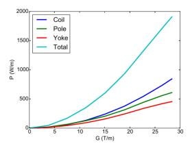
Figure 5: Total power loss in the quadrupole per m length.
