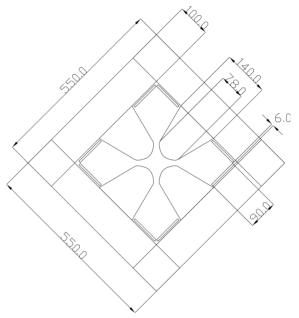
Figure 2: Magnet Geometry (all dimensions in mm).
