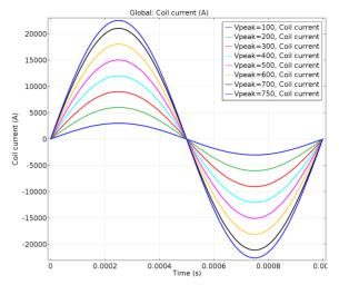
Figure 7: Current in one excitation coil as a function of applied voltage.
