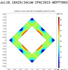
Figure 3: Core loss (in W/kg) in the pole of the magnet (left figure) and the return yoke (right figure) at a frequency of 1 kHz.
