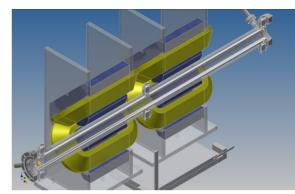
Figure 3: Vertical kicker inside a quadrupole doublet.
