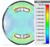
Figure 5: Transverse cross-section of electric field (vert. kicker).
