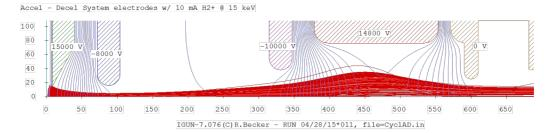
Figure 4: IGUN simulation of beam extraction and matching to RFO.
