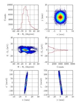
Figure 3: Phase Spaces of the RFQ output beam.
