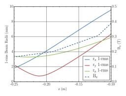
E Figure 5: The 1-rms bunch radii for the beam traveling from the exit of the RFQ to the entrance of the spiral inflector. The residual axial magnetic field of the cyclotron is plotted on the secondary axis.
