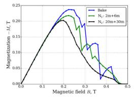
Figure 2: DC Magnetization of niobium samples as a function of external magnetic field at 2 K.
