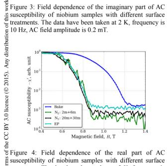
susceptibility of niobium samples with different surface treatments. The data have been taken at 2 K, frequency is
