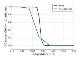
Figure 1: Real part of the linear AC susceptibility measured near zero-field transition temperature of the niobium samples. All considered samples have critical temperature about 9.25 K. The width of transition region depends on existence of normal conducting fractions at the surface of the superconductor.
