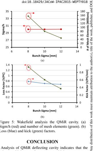
Figure 5: Wakefield analysis the QMiR cavity. (a) Sigm/h (red) and number of mesh elements (green). (b) Loss (blue) and kick (green) factors.
