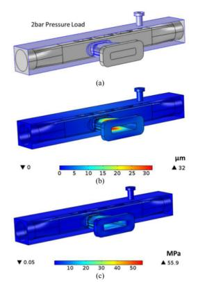
Figure 2: Frequency sensitivity to pressure fluctuation df/dP of the QMiR cavity. (a) Boundary conditions. b) Displacement in  $\mu$ m. (c) Von Mises stresses in MPa along the structure.
