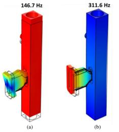
Figure 4: Modal analysis of the OMiR cavity showing lowest two mechanical resonances. (a) 146.7 Hz mode. (b) 311.6 Hz mode.
