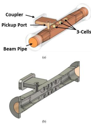
Figure 1: Geometry of the quasi multimode resonator. (a) RF domain is highlighted. (b) Section of the cavity with the Niobium walls highlighted.
