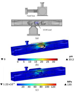
Figure 3: Investigation of frequency sensitivity to tuning forces for the QMiR structure. (a) Cavity with boundary load of 15 kN. (b) Resultant displacement in  $\mu$ m. (c) Resultant Von Mises stresses in MPa along the structure.
