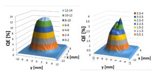
Figure 1: QE maps of Cathode #198 (Cs<sub>2</sub>Te) as newly produced (left) and used in the RF photoinjector (right).
