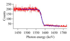
Figure 3: Measured CBS spectrum at 1.3 GeV with fit to determine the Compton edge energy. Signal integrated over 120 seconds.
