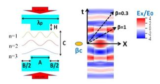
Figure 2: Illustration of the first, second and third spatial harmonic mode in one grating period, driven from opposite sides by laser.
