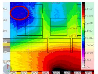
Figure 6: Prompt radiation levels around the target area and the proposed electronics positions in TT61 (red circle). The radiation levels are shown in fluence/cm2 (hadrons > 20 MeV) and for  $3.7 \times 10^{12}$  protons impinging on a thick target.
