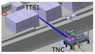
Figure 5: Integration study of a HiRadMat experiment placed on the position B. The adjacent tunnel TT61 hosts the sensitive electronics e.g. of the high-speed cameras, where the optical path passes through the recently installed feed-throughs.
