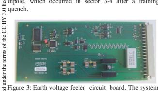
Figure 3: Earth voltage feeler circuit board. The system  $\frac{1}{2}$  can measure voltages in the range of  $\pm 2$  kV with a  $\stackrel{\text{B}}{\rightarrow}$  resolution better than 1 mV.
