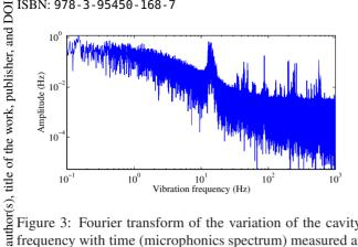
Figure 3: Fourier transform of the variation of the cavity frequency with time (microphonics spectrum) measured at T = 4 K,  $E_{acc} = 1$  MV/m and a pressure of 1 bar.
