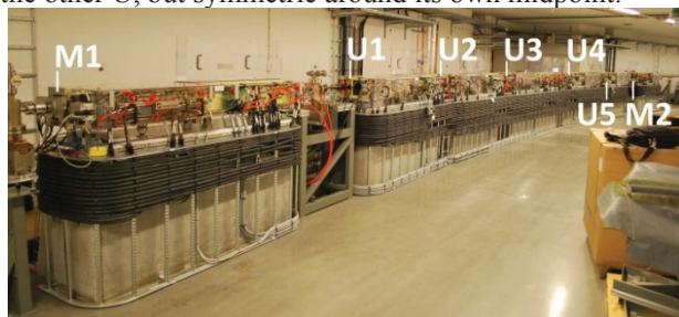
Figure 2: Achromat 04 in the 3 GeV ring, fully assembled.
