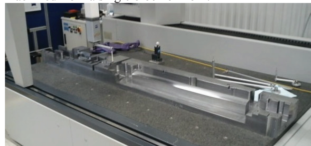
Figure 3: U4/U5 yoke bottom half undergoing 3D mechanical measurement.
