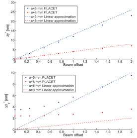
Figure 6: Linear approximation and PLACET simulations of the orbit displacement (top) and beam size growth (bottom) as a function of the beam offset for a=5 mm and a=8 mm.
