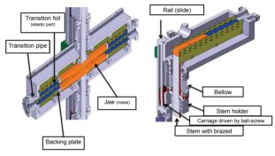
Figure 1: Detailed 3D mechanical design.
