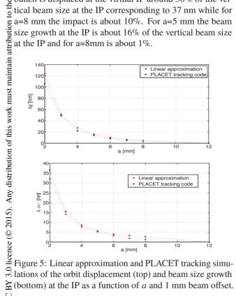
BY (bottom) at the IP as a function of a and 1 mm beam offset. 5
