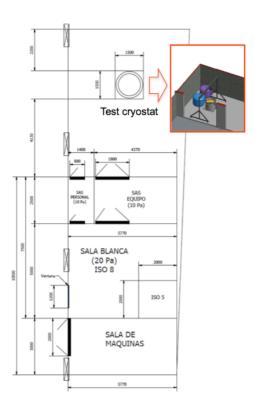
Figure 2: Sketch of the clean room build for RF cavity assembly and test.
