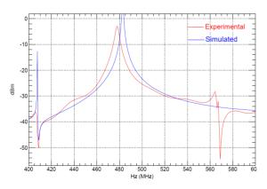
Figure 3: RFQ frequency test at the RF lab.
