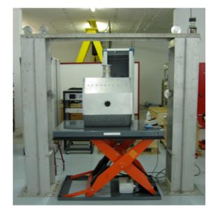
Figure 1: Bead pull system and cold model of RFQ in aluminium.
