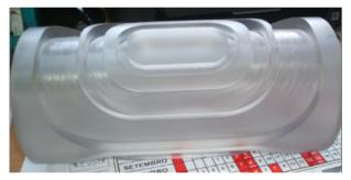
Figure 5: Prototype of a magnet support on which coppermade coil blocks will be winded.
