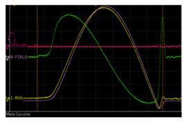
Figure 6: Image from magnetic measurements. Yellow trace is the current pulse, green is the induced voltage pulsed and purple is the integrated magnetic field.
