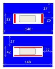
Figure 2: Cross section sketch of the HOR (upper) and VER (lower) pinger magnet. Dimensions in mm.
