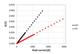
Figure 7: Magnetic field linearity with current pulse.
