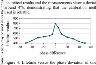
Figure 4: Lifetime versus the phase deviation of one of the cavities. The maximum is gotten for in phase Content operation.
