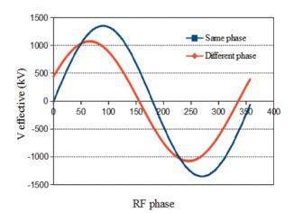
Figure 2:  $\overline{V_{eff}}$  when RF phases between the three cavities are the same and when  $\phi_1 = \phi_2 \neq \phi_3 = \phi_1 + 80$ .
