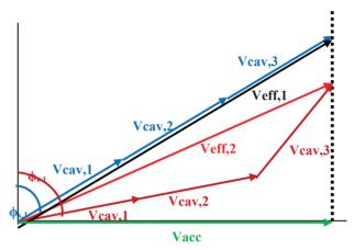
Figure 1: The effective voltage, Veff,1, is the sum vector of three cavity voltage in phase and Veff.2 is the sum when two cavities are in phase and one not  $\phi_{s,1} = \phi_{s,2} \neq \phi_{s,3}.$
