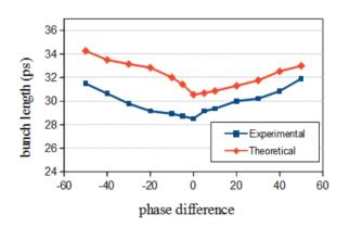
Figure 6: Bunch length versus the phase deviation of one of the cavities. The maximum is gotten for in phase operation.
