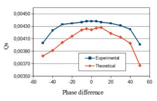
Figure 5: Synchrotron tune versus the phase deviation of one of the cavities. The maximum is gotten for in phase operation.
