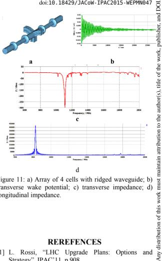
Figure 11: a) Array of 4 cells with ridged waveguide; b) transverse wake potential; c) transverse impedance; d) longitudinal impedance.
