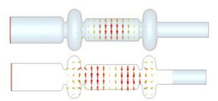
Figure 7: Distribution of electric field of trapped modes.
