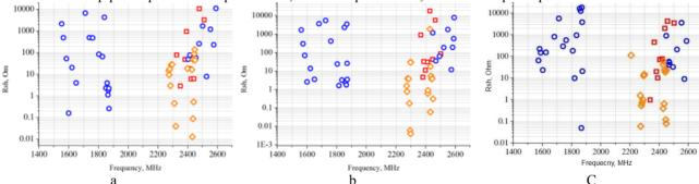
Figure. 6. R<sub>sh</sub> for 9-cell elliptical structure with a) fluted beam pipes; b) ridged beam pipes; c) corrugated beam pipes Square – monopole waves, circle – dipole waves, diamonds – quadrupole waves.
