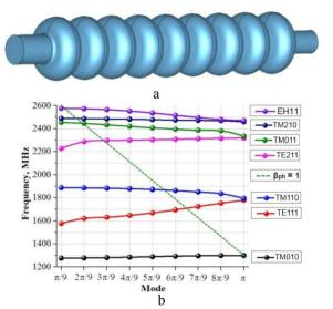
Figure. 1.Genearal view (a), dispersion characteristics (b), for 9-cell cavity with cylindrical beam pipes
