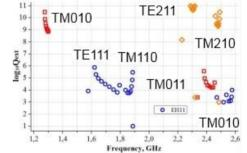
Figure. 2. Q<sub>ext</sub> for 9-cell cavity with cylindrical beam pipes
