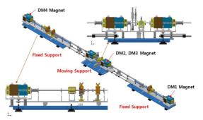
Figure 3: 3D modelling of BC support system.
