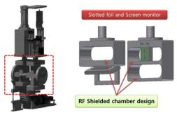
Figure 8: Design of the RF shielded chamber.
