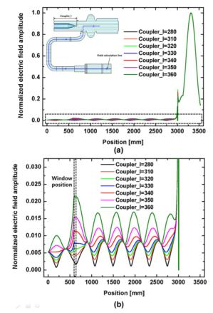
Figure 2: (a) Changes that occurred in the simulated normalized electric field amplitude due to Coupler\_l and (b) the magnified graph of the dotted-box region shown.
