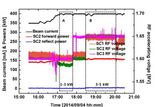
Figure 4: The beam current, RF voltages, forward power and reflect power measured during the top-up operation test with the beam current of 400 mA.
