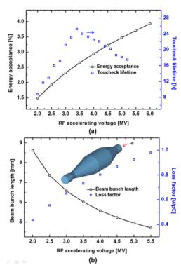
Figure 1: (a) Calculated energy acceptance and Touschek lifetime and (b) the beam bunch length and the loss factor of the PLS-II SC taper section. The three-dimensional modeling of the SC taper section is shown in the inset.
