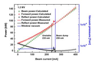
Figure 3: The beam power, forward power, and reflect power calculated, and the forward power, reflect power measured, and the window vacuum pressure of SC2 in the beam current domain during the beam store test with the RF accelerating voltage of 1.2 MV.
