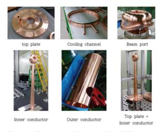
Figure 4: The picture of the parts of the QWR cavity.
