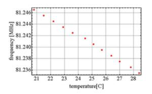
Figure 7: The measured resonance frequency as a tempera ture.
