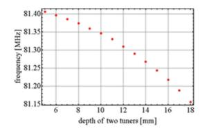
Figure 9: The measured resonance frequency as a function of two tuners depth.
