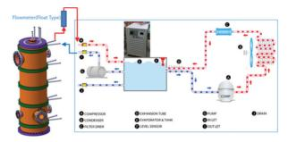
Figure 6: Schematic drawing of the cooling channel test.
