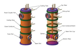
Figure 1: Drawing of the QWR cavity in MEBT of RAON.
