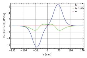
Figure 2: Electric field profile along the beam axis.
