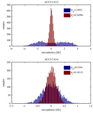
Figure 6: Histograms of the static detuning and one-step ahead prediction error of the proposed method for cavities 2 and 4 in the module ACC5 ( $\sigma_{\Delta f}$  - standard deviation of the static detuning,  $\sigma_{\varepsilon}$  - standard deviation of the one-step prediction error).
