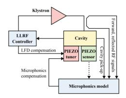
Figure 1: Block diagram of the proposed microphonics compensation method for a linac operating in pulsed mode.
