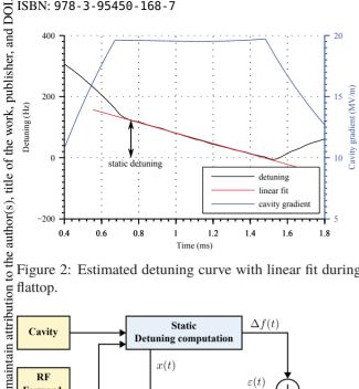
Figure 2: Estimated detuning curve with linear fit during flattop.
