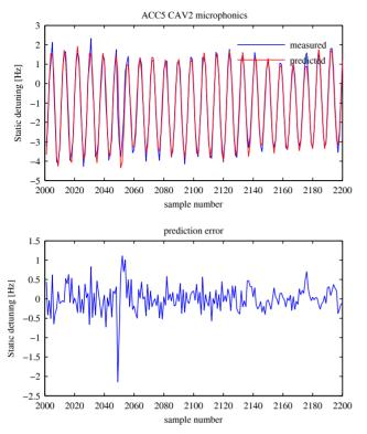
Figure 5: Static detuning and one-step prediction error at the FLASH ACC5 module cavity 2.
