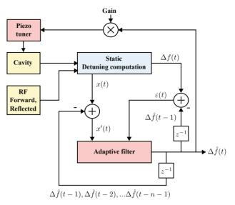
Figure 4: Schematic diagram of the microphonics compensation strategy.
