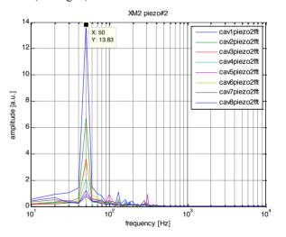
Figure 1: Microphonics measurement at XM-2 module.
