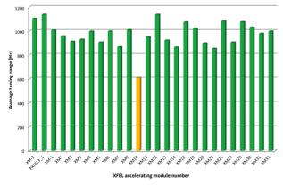
Figure 3: The cavity tuning range measurement of XFEL modules using piezo actuators.
