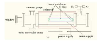
Figure 2: Schematic diagram of DC magnetron sputtering coating system.
