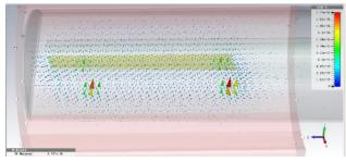
Figure 3: The electric displacement vector distribution in the case of ceramic pillars as cathode brace, during glow discharge.
