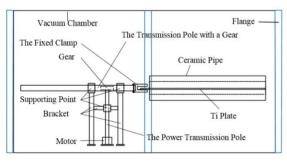
Figure 5: Schematic diagram of single motor drive.
