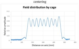
Figure 5: Field  $(E_Y)$  distribution of s-band deflecting structure.
