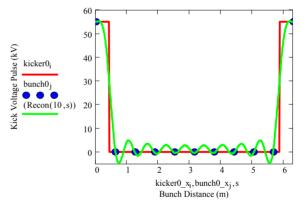
Figure 2: Ideal kicker voltage pulse (red) and bunch train scheme (blue) to kick every  $10^{th}$  bunch, and the reconstructed kicker pulse with the first 10 harmonic modes (green).
