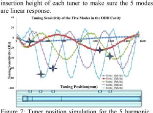
Figure 7: Tuner position simulation for the 5 harmonic modes cavity with a small cylinder perturbation.
