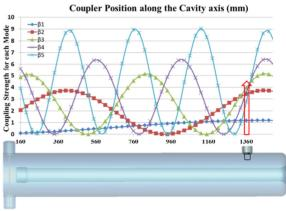
Figure 8: Loop coupler position optimization.
