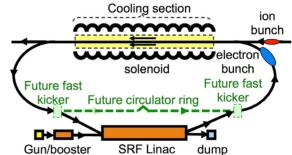
Figure 1: A schematic drawing of a bunched beam cooler based on an ERL, with bypass circulator ring connection in green.
