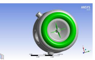
Figure 6: Stiffeners on cavity end wall (highlighted green colour).
