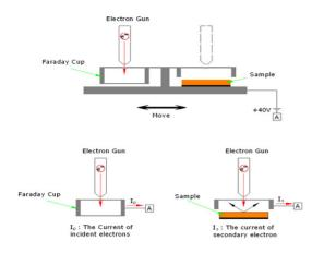
Figure 2: Schematic diagram of the Faraday cup.
