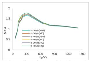
a) Stainless steel, emission current: 1µA, gird voltage: 9V focus voltage: 100V, 1st anode voltage: 100V.
