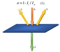
Figure 1: The SEY measurement principle.
