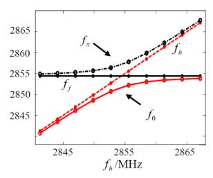
Figure 5: Variation of  $f_0$  and  $f_{\pi}$  with half-cell frequency for a constant full-cell frequency.
