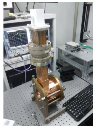
Figure 6: Experiment setup for RF gun measurement.
