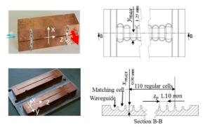
Figure 2: Sketch of W-band wakefield structure.
