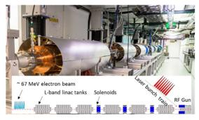
Figure 1: Layout of AWA drive beam line.
