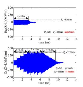
Figure 3: RF output simulation results from CST.
