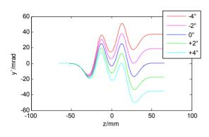
Figure 6: Vertical deflection along z axis with different phases.
