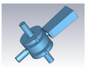
Figure 7: The RF deflector with coupler.
