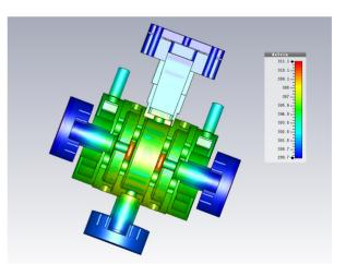
Figure 9: Thermal simulation result of the cavity.
