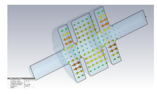
Figure 2:  $\pi$ -mode needed in the RF cavity.
