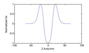
Figure 4: Normalized  $H_x$  along z axis.
