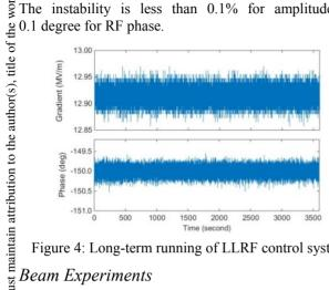
Figure 4: Long-term running of LLRF control system.
