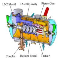
Figure 1: Schematic view of the DC-SRF photoinjector.
