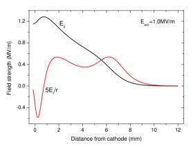
Figure 4: Simulated longitudinal and radial electric fields along the gun axis.
