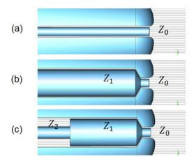
Figure 7: (a) The simple coaxial line structure. (b)The coaxial line structure with once diameter changing. (c)The coaxial line structure with twice diameter changing.
