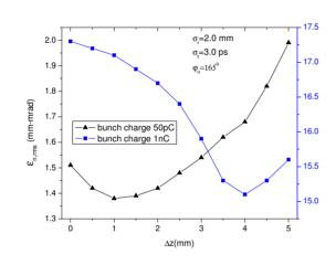
$\frac{1}{2}$  Figure 6: The optimum  $\Delta z$  for best transverse emittance is affected by different beam parameters. Q
