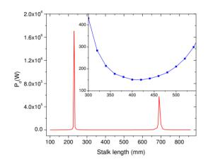
Figure 2: The magnitude of the power dissipation versus stalk length.
