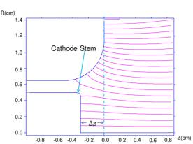
Figure 3: Close view of the field pattern near the cathode for the 32MHz QWR cavity.
