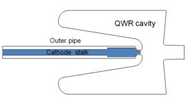
Figure 1: The schematic of 325MHz QWR cavity and the cantilevered cathode stalk.
